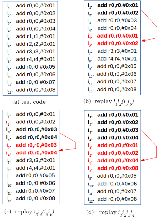
Fig. 3. Test code and replay fault definitions: (a) test code, (b) replay i_1i_2(i_5i_6) , (c) replay i_3i_4(i_5i_6) , (d) replay i_1i_2i_3i_4
