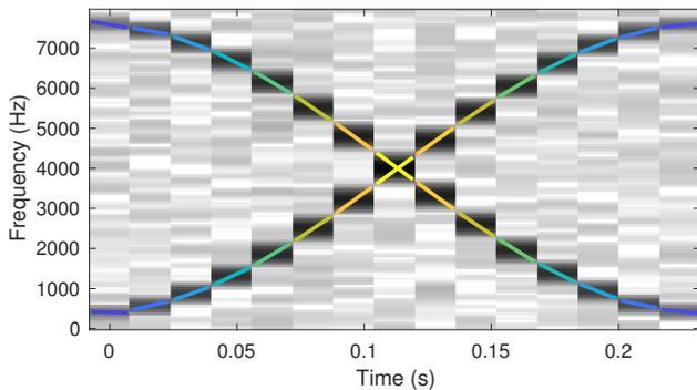
(b) NLR accurately resolves and estimates the two cosine FM sounds from a noisy signal, even at 0.12 seconds where they share the same 4kHz spectral peak.
