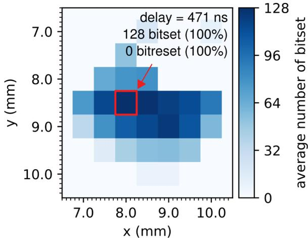
Figure 5: Sensitive area to EM fault injection
