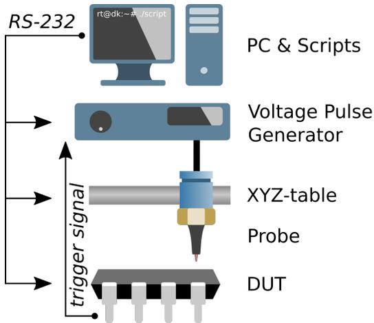
Figure 2: Schematic of the EM pulse injection setup
