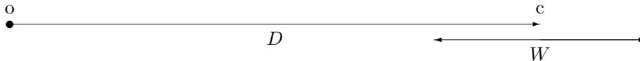
Fig. 1. One-dimensional single-shot movement paradigm settled by Fitts [2]. Starting at origin o , one moves towards the center c of the target as fast as possible.
