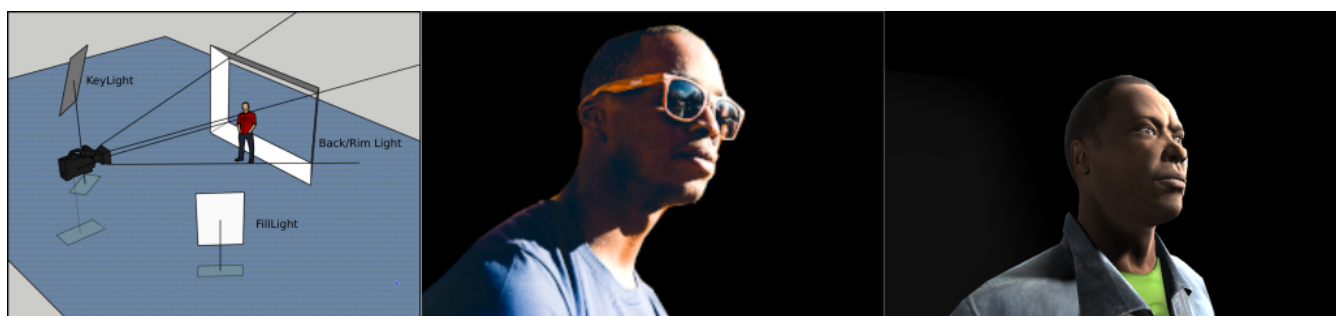
Figure 1: The 3-point-lighting technique (on the left) is a classical cinematic rule to place lights around a subject. Playing with the lights position, size, and flux considerably impacts the aesthetics and atmosphere of a scene (in the middle). We propose a technique that automatically computes the parameters of a 3-point-lighting setup made of area lights, given the reference image in the middle, to generate the image on the right in a virtual environment.
