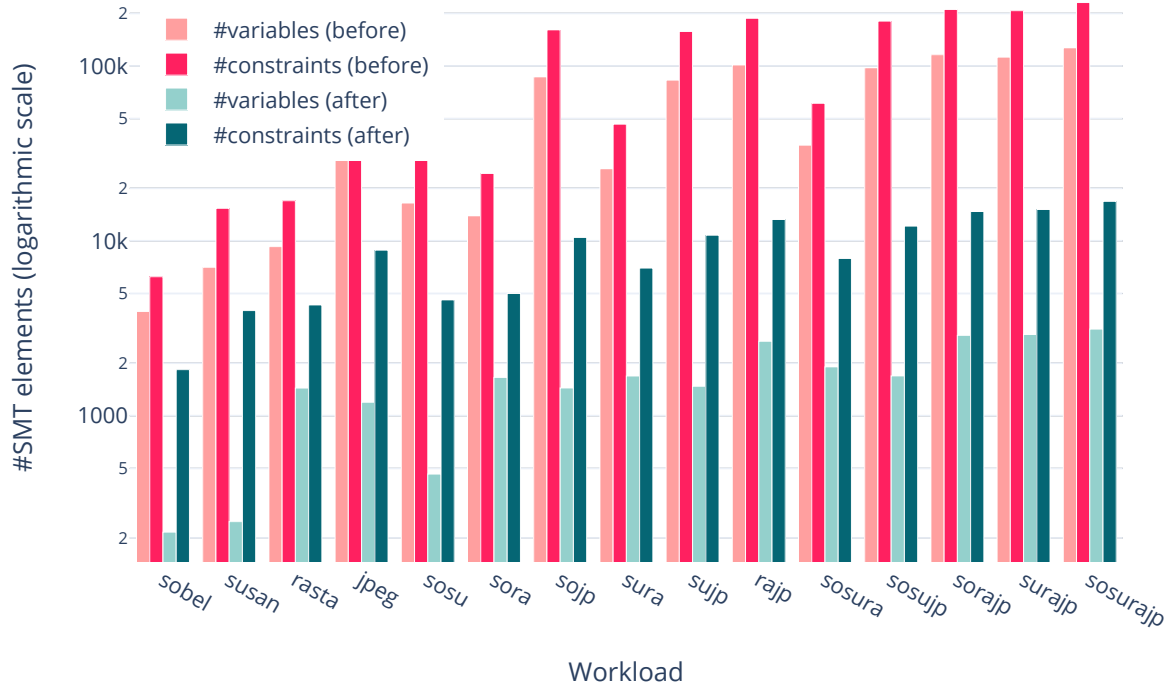
Figure 4.7: Comparison of the size of the SMT model, as the number of created variables and constraints, before and after applying the reduction method, as a function of different workloads.
