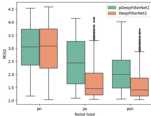
**Fig. 2:** Box plot featuring the PESQ for DeepFilterNet2 and pDeepFilterNet2 (unified encoder version) for different noise types: primary speaker + noise (pn), primary speaker + secondary speaker (ps), primary speaker + secondary speaker + noise (psn).
