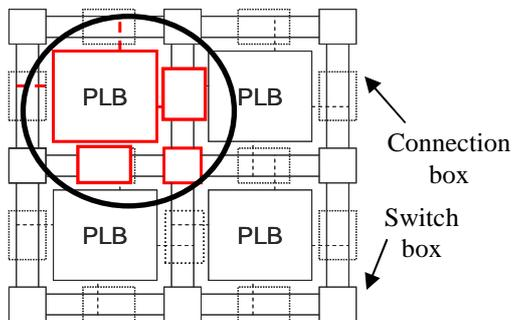
Figure 1: e-FPGA architecture.
