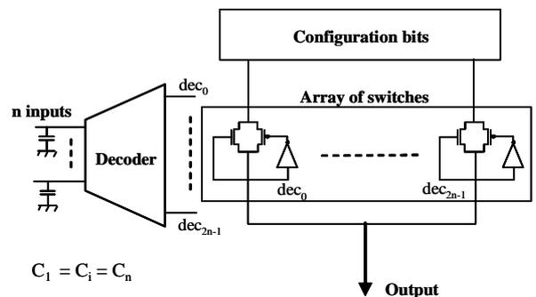
Figure 4: Balanced LUT implementation.
