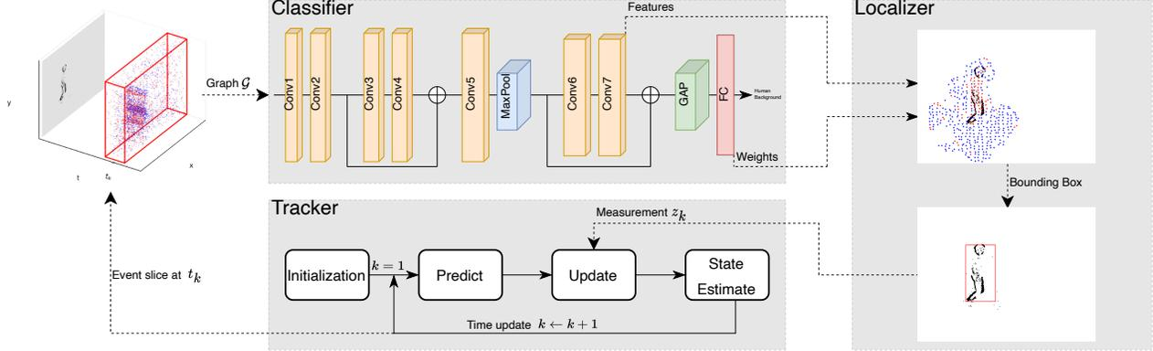
**Fig. 1.** Our proposed single human tracking framework: The *Human Classifier* is a binary classifier that predicts whether the event graph contains a human or background object. In the case of a predicted human label, the *Human Localizer* produces a bounding box which encodes the location of the human. The *Human Tracker* deploys a Kalman filter for tracking the human which models the generated bounding box as a sensor measurement.
