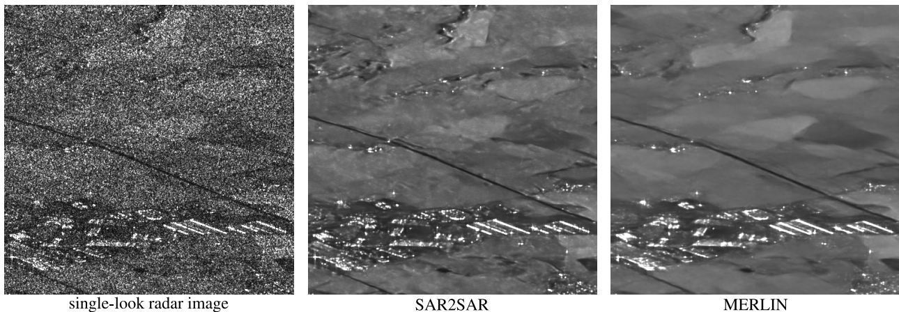
Figure 6 Results on Sentinel-1 TOPS data. Left: the speckle corrupted amplitude image. Center: the image filtered with SAR2SAR. Right: estimation produced with MERLIN.
