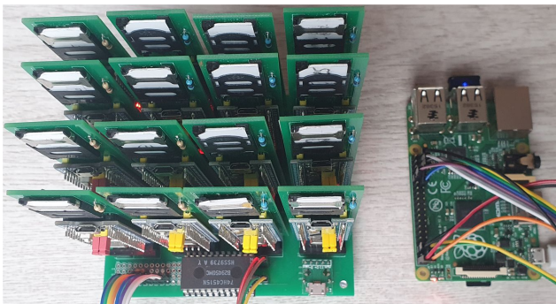
Fig. 10. A personal HSM. Grid of secure element with I 2 C connectivity (left) and host system (Raspberry Pi, right)
