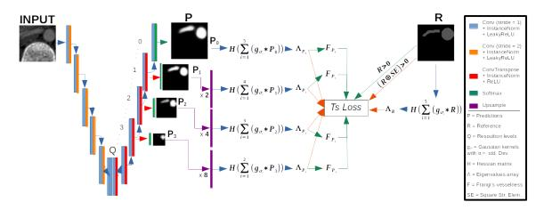
Figure 7: Tubular structures loss function (TsLoss) pipeline. The function is composed of two loss terms, one based on the eigenvalues  $\Lambda$  of the Hessian matrix calculated for every voxel of the filtered segmentation masks, and another based on the F Frangi's vesselness function (Frangi et al., 1998) calculated from these eigenvalues. The TsLoss term is applied in deep supervision for the first 4 resolution levels, together with voxel-wise loss functions. See text for details.
