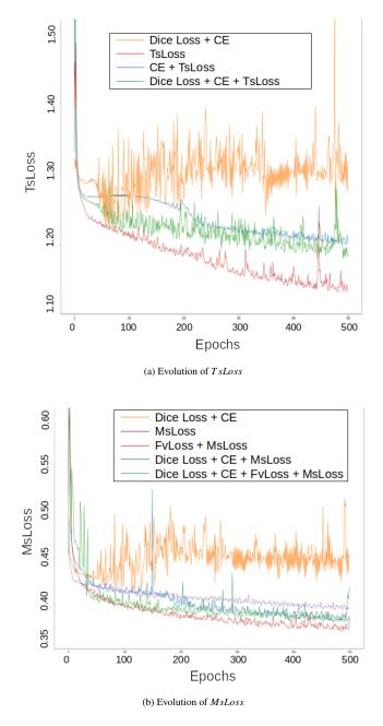
Figure 12: Evolution of proposed losses during training for different loss functions combinations.
