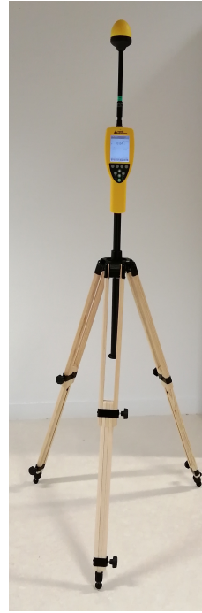
Figure 2. NBM-550 broadband measurement system
