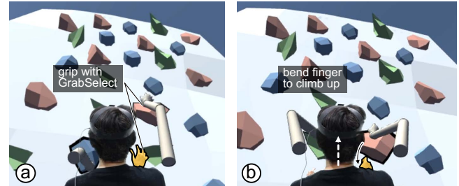
Figure 8: (a) The user selects a grip with GrabSelect . (b) While gripping, the user bends the finger to pull the body upwards and create a vertical displacement in VR.
