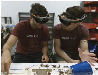
Figure 2. A dyad pair interacting with the system while seeing AR through Microsoft Hololens headsets.
