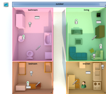
Fig. 10: The iCasa GUI showing the basic setup for our experiments: four rooms equipped with a presence sensor triggering heating and lighting, and a thermometer.
