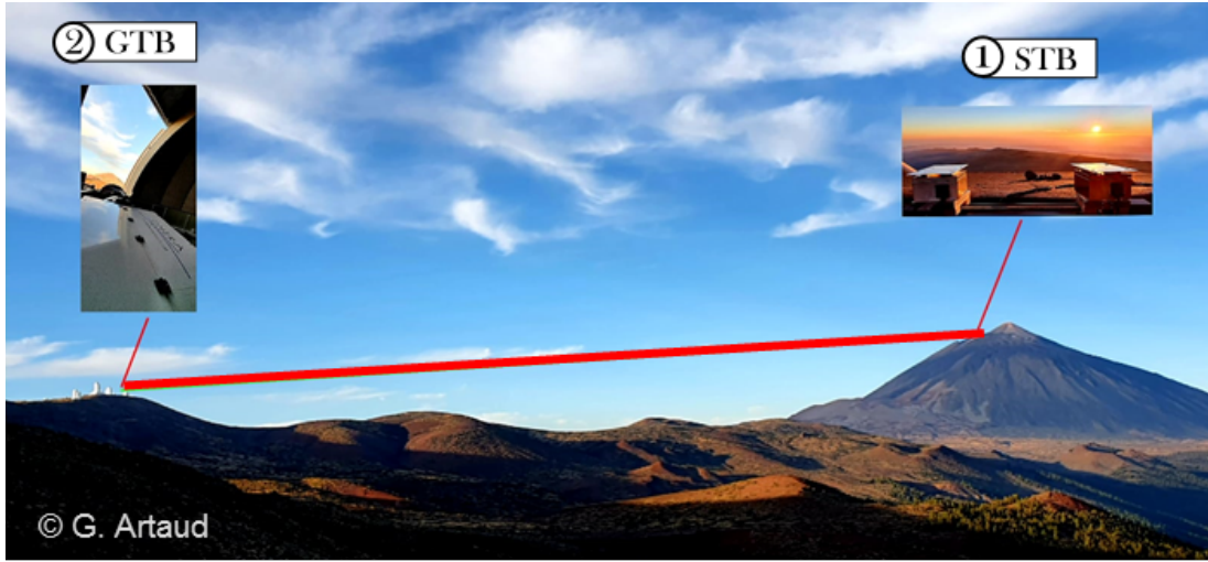
Fig. 1. Picture of the 13.2 km line of sight between the OGS Dome (GTB) and the satellite emulator on top of the Teide mountain (STB). Credits Geraldine Artaud (CNES).
