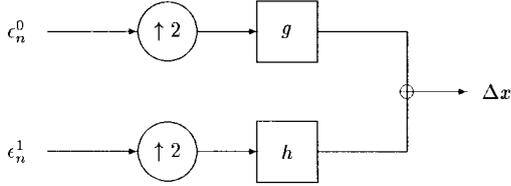
Fig. 4. Reconstruction error. Only one iteration of a 1-D signal is considered.  $\epsilon_n^0$  and  $\epsilon_n^1$  are quantization errors.  $\Delta x$  is the reconstruction error,  $g$  and  $h$  are the set of the filter coefficients.
