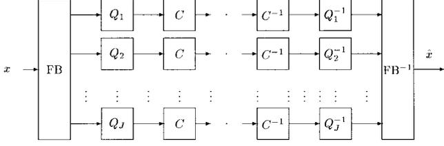
Fig. 3. Filterbank compression scheme. The encoding part uses an octave-band separable filterbank (wavelet transform) iterated  $J$  times on the lowpass filter which splits the input image into  $(3J + 1)$  subimages. These subimages are then quantized and losslessly encoded (using Huffman coding). The synthesis part reconstructs the approximate signal  $\hat{x}$ .
