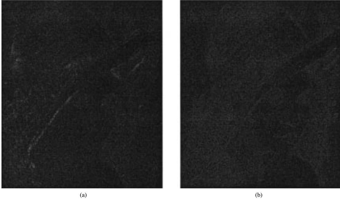
Fig. 10. Error images between the original image (Lena,  $512 \times 512$ ) and the reconstructed ones after a compression to 1.4 b/pixel (global Huffman coding) with  $L^2$  and  $L^\infty$  criteria. (a) Error image obtained in the  $L^2$ -norm context. (b) Error image obtained with  $L^\infty$ -norm. The errors in (a) are higher and more concentrated on the edges than in (b).
