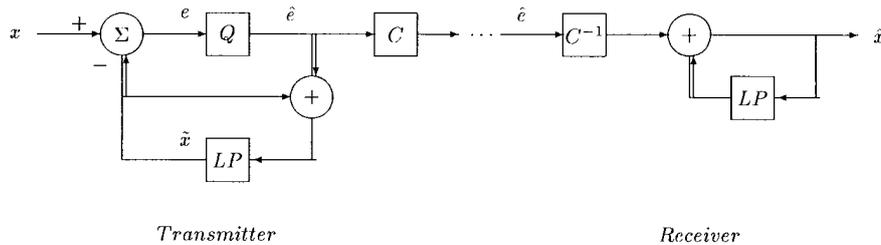
Fig. 1. DPCM block diagram. The transmitter includes the receiver to ensure identical prediction on both sides.  $LP$  denotes the predictor. The prediction error is quantized, encoded (global Huffman coding) and transmitted. The receiver reconstructs the approximate signal  $\hat{x}$ .
