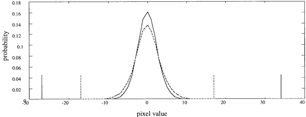
Fig. 9. Histogram of the errors with  $L^2$  and  $L^\infty$  criteria in the reconstructed Lena images at the bit rate of 1.4 b/pixel (given by a global Huffman coding) using the MSE-criterion (solid curve) and the  $L^\infty$ -criterion (dashed curve). The vertical lines (dashed lines for  $L^\infty$  and solid lines for  $L^2$ ) show the minimum and maximum error values in both cases. As expected, the maximum error is higher with  $L^2$ -criterion than with  $L^\infty$ -criterion.
