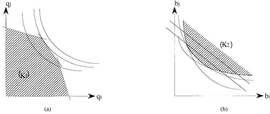
Fig. 6. Equivalent constrained optimization problems. (a) Problem  $(P_1)$  has a convex cost function and linear constraints delimiting the feasible domain  $(K_1)$ . (b) Problem  $(P_2)$  has a linear cost function and convex constraints, the feasible domain is  $(K_2)$ . It is easily seen from  $(P_1)$  the optimum solution is on the boundary of  $(K_1)$  or  $(K_2)$ .
