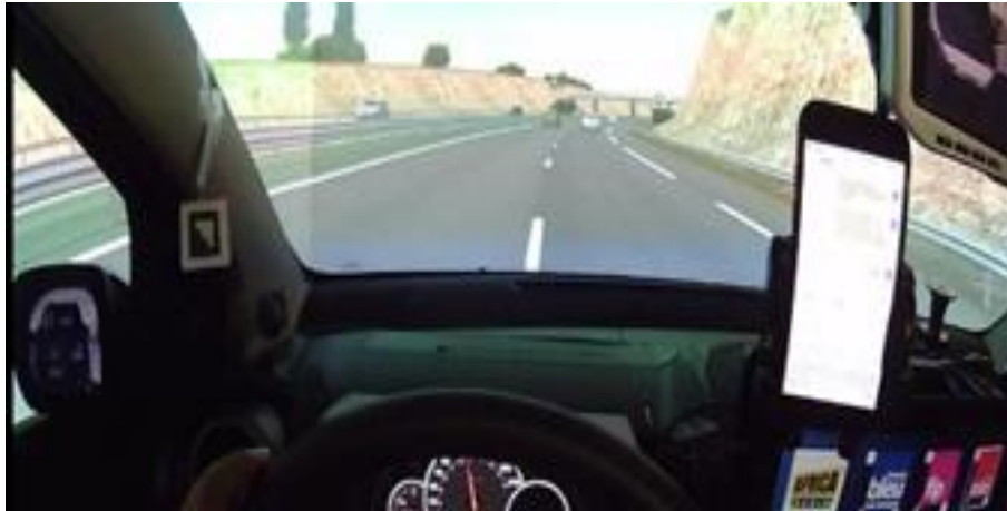
Fig. 1. Event 1 (EV1) Incidental loss of assistance in a high-speed turn (130 km/h)
