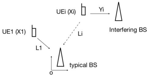
Fig. 1: System model in uplink OMA scheme.
