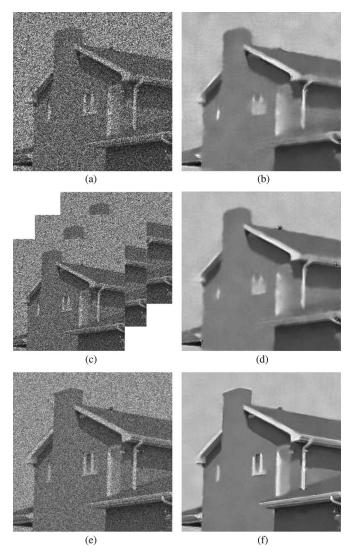
Fig. 2. Denoising results of synthetic images with multiplicative speckle noise (left: input noisy images; right: denoising results). (a) 1-look noisy image. (b) Method i 1-PPB result of (a); SNR: 10.79. (c) Three 1-look noisy multitemporal images. (d) Method ii T-PPB result of (c); SNR: 11.62. (e) Temporal mean of (c) (a 3-look noisy image). (f) Method iii M-PPB result of (e); SNR: 13.81.
