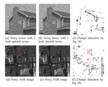
Fig. 5. Change detection by the KL divergence and the GLR criterion. (a) and (b) Noisy house images with 1-look speckle noise. (c) Change detection results between (a) and (b). (d) and (e) Noisy SAR images; the red rectangles denote the changes between (d) and (e). (f) Change detection results between (d) and (e). Changes in red rectangles have been found out in detection results.
