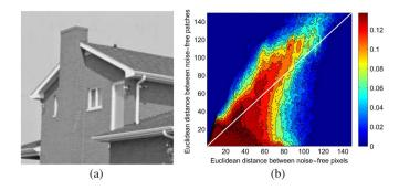
Fig. 1. Two-dimensional histogram of the Euclidean distance between noise-free patches K and noise-free pixels. The ideal case (the assumption that similar patches have similar central pixels [29]) is shown on the white line. (a) Test image house. (b) Two-dimensional histogram of the Euclidean distance.
