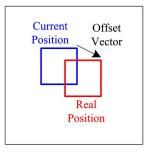
Fig. 6. Assumption of image registration. In the intensity image registration, all pixels in a small patch share the same offset to their real position.
