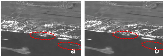
Fig. 6: Improved temporal filtering with a super-image obtained by denoising the geometric mean: the speckled image at the date t = 11 (shown in Fig.4(a)) is restored by RABASAR using a super-image obtained from (a) the arithmetic mean, or (b) the geometric mean. Note the reduction of artifacts in the circled area with the geometric mean.
