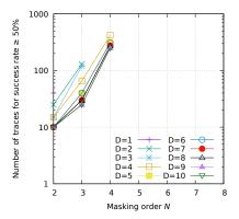
**Fig. 7** Number of traces necessary for  $SR \ge 50\%$  for correct MS-DSM on n = 4 bits (when  $\sigma = 1$ ), as a function of the masking order N = d + 1, for several sub-trace dimensionalities D
