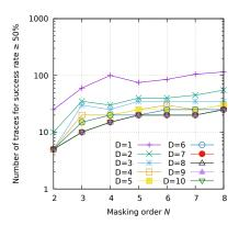
**Fig. 6** Number of traces necessary for  $SR \ge 50\%$  for incorrect MS-DSM on n = 4 bits (when  $\sigma = 1$ ), as a function of the masking order N = d + 1, for several sub-trace dimensionalities D
