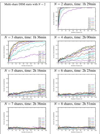
**Fig. 11** Attacks on  $D=1,\ldots,10$  samples for noise  $\sigma=1.0$ , and various number of shares (for 100 attacks) against (correct, see App. A.2) Multi-shares DSM on PRESENT (n=4 bit)
