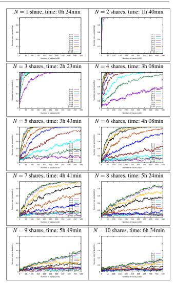
**Fig. 9** Attacks on  $D=1,\ldots,10$  samples on Boolean Masking of PRESENT (n=4 bit) for noise  $\sigma=1.0$ , and various number of shares (for 100 attacks)
