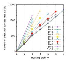
**Fig. 4** Number of traces necessary for  $SR \ge 50\%$  on n = 8 bits (when  $\sigma = 1$ ), as a function of the masking order N = d + 1, for several subtrace dimensionalities D
