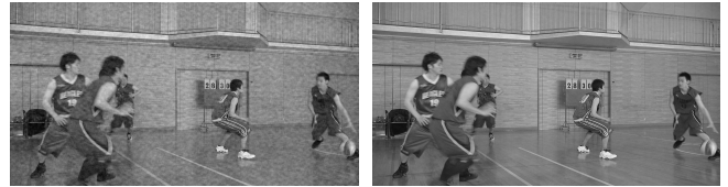
Fig. 1: Visual quality comparison for the BasketBall Drive sequence (frame No.90), GoP-size = 32, no compression applied. Left: strong snow-effect (CSNR=0dB), right: slight snow-effect (CSNR=15dB).
