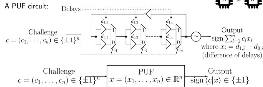
The PUF parameter  $x$  is **uncontrollable**: it depends on the manufacturing process and varies from one circuit to another ("static randomness").
