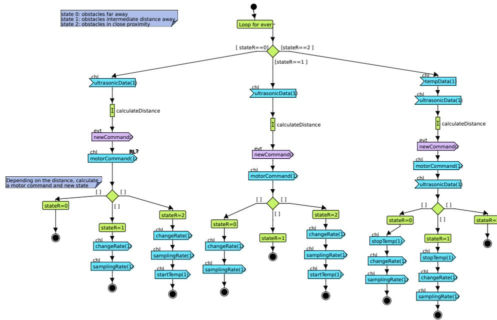
Figure 5. Activity diagram of the main control
