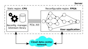
Fig. 1. The architecture of a modern FPGA-based server.
