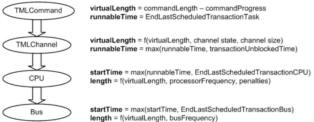
Fig. 5. Data flow of a transaction
