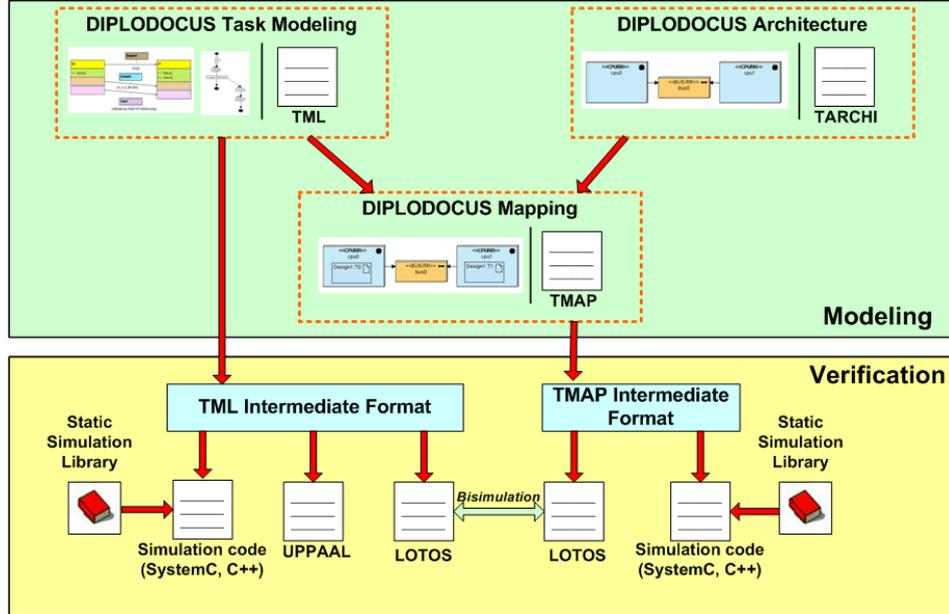
Fig. 2. Modeling and verification capabilities of TTool
