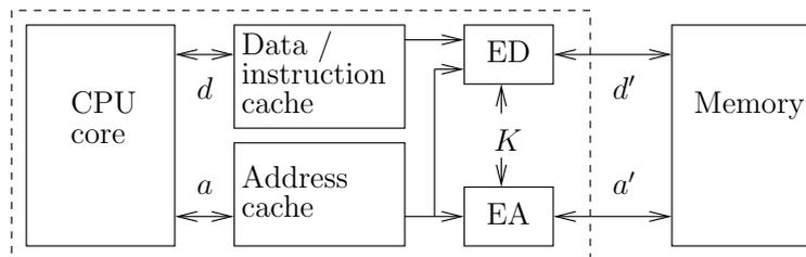
**Figure 1:** Bus-encryption processor (dashed box) plus external memory.
