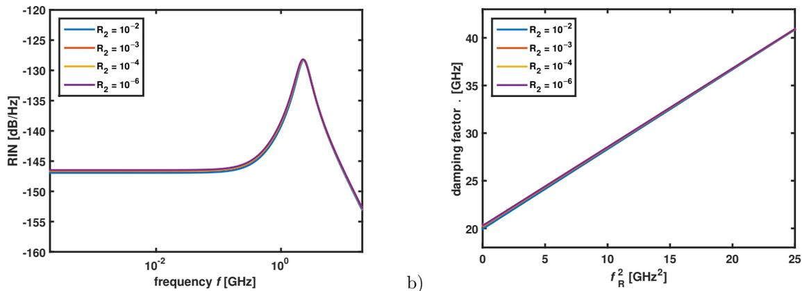
Figure 7. Impact of the AR coating impairment on the a) RIN and b) damping factor assuming a power reflectivity  $R_2$  ranging from  $10^{-2}$ ,  $10^{-3}$ ,  $10^{-4}$ , to  $10^{-6}$ . The length of the EC is fixed to  $\ell_{\text{ext}} = 6$  cm.
