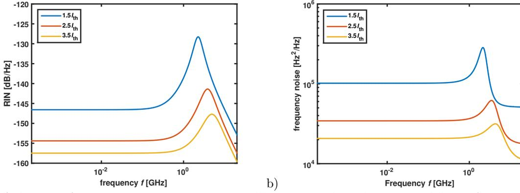
Figure 5. a) RIN and b) FN spectra calculated for three different normalized bias currents  $1.5 \times I_{th}$  (upper blue curves),  $2.5 \times I_{th}$  (center red curves), and  $3.5 \times I_{th}$  (lower yellow curves). The length of the EC is fixed to  $\ell_{ext} = 6$  cm.
