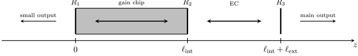
Figure 1. The external cavity (EC) laser has an EC length of  $\ell_{\text{ext}}$  and a round trip time of  $\tau_{\text{ext}}$  within mirror reflectivities  $R$ . The light output of the gain chip at the rear facet (reflectivity  $R_1$  at  $z = 0$ ) is much smaller than the main output at  $z = \ell_{\text{int}} + \ell_{\text{ext}}$ . In this work, mirror 2 with reflectivity  $R_2$  is simulated with an anti-reflection coating in EC operation.
