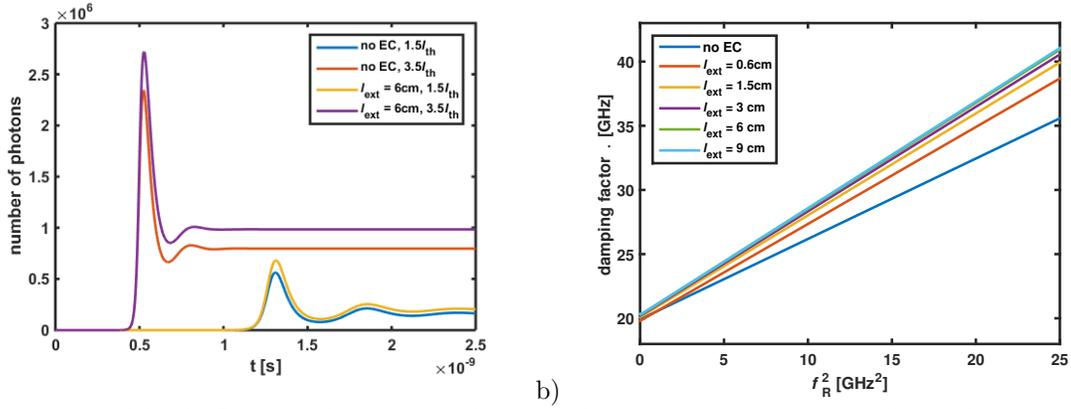
Figure 4. a) Turn-on delay b) Damping factor  $\gamma$  as a function of the squared relaxation oscillation frequency  $f_R^2$  for no EC (dark blue), and different EC lengths: 6 mm (red), 1.5 cm (yellow), 3 cm (violet), 6 cm (green), and 9 cm (light blue).
