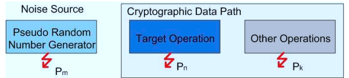
Figure 1: : Increasing resistance to attacks by adding high noise level
