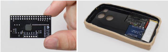
Figure 11. Left. Open Hardware Mutual Capacitance breakout Right. Smartphone case prototype hardware.
