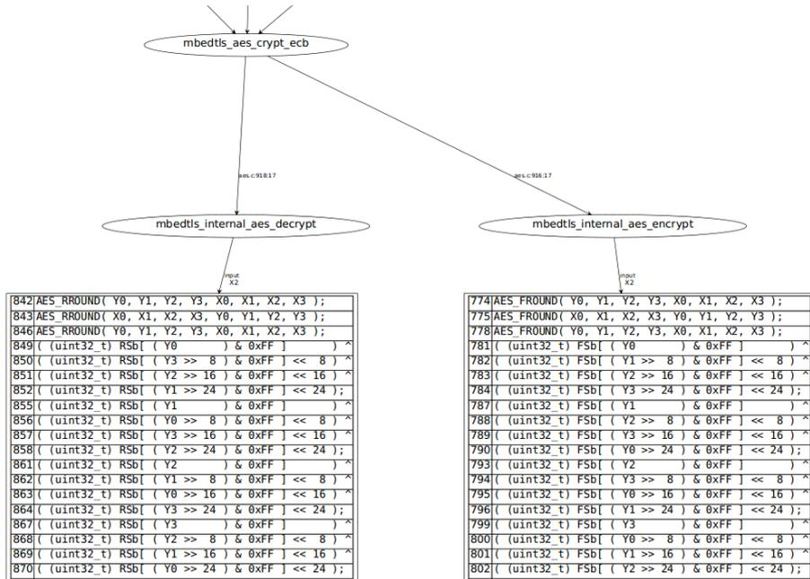
Fig. 9. AES leakage tracking and code location
