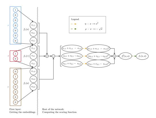
**Fig. 4.** Graphical representation of the TransE Model (with 2-norm) applied to the fact *marriedTo*(*Barack*,*Michelle*) for Figure 1, with  $s = (1\ 0\ 0\ 0\ 0\ 0\ 0)^T$ ,  $o = (0\ 1\ 0\ 0\ 0\ 0\ 0)^T$  and  $r = (1\ 0)^T$ .
