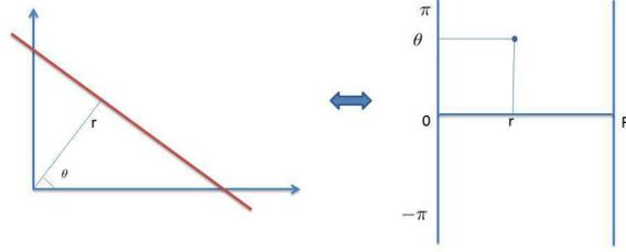
Figure 1: Line parametrization.
