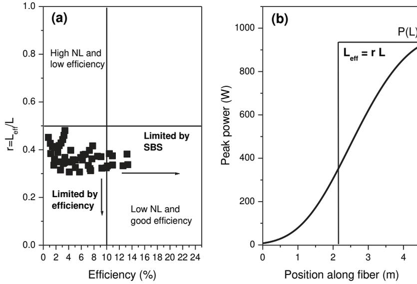
**Fig. 12.** (a) Modeling results of the variation of  $r = L_{\text{eff}}/L$  for various input peak power and pump power fiber amplifiers based on the Thulium doped fiber (cf. Table 1) as a function of the efficiency (output average power divided by input pump power) achieved for various fiber lengths, (b) chart showing an example of the power distribution in the Thulium doped fiber amplifier.
