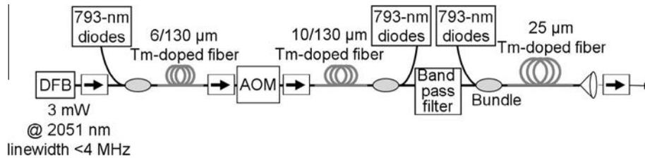
Fig. 6. Three stages amplifier layout. AOM, acousto-optic modulator.
