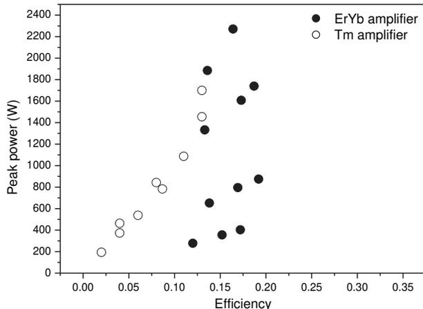
**Fig. 14.** Modeling results of the variation of output peak power for various input peak power and pump power fiber amplifiers based on the Erbium–Ytterbium codoped fiber (full disks) and Thulium doped fiber (open disks) (cf. Table 1) as a function of the efficiency achieved for various fiber lengths.
