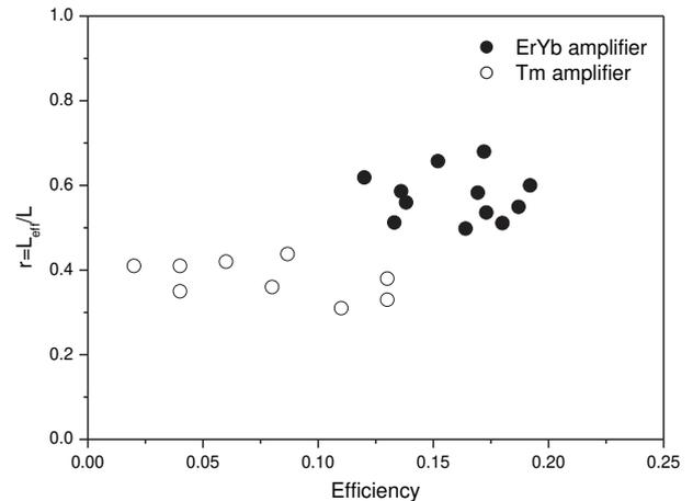
**Fig. 13.** Modeling results of the variation of  $r = L_{\text{eff}}/L$  for various input peak power and pump power fiber amplifiers based on the Erbium-Ytterbium co-doped fiber (full disks) and Thulium doped fiber (open disks) (cf. Table 1) as a function of the efficiency achieved for the lengths indicated in Table 1.
