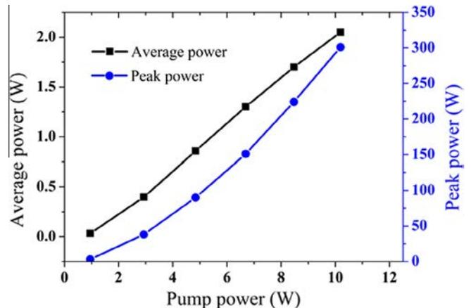
Fig. 3. Average power and peak power vs. pump power in the power amplifier stage. SBS limits the extractable energy.
