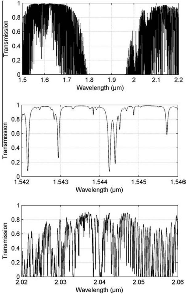
**Fig. 1.** Atmospheric transmission of a 10 km horizontal path on ground (standard atmosphere, no aerosol). Top: 1.5–2.2  $\mu\text{m}$  transmission, middle: 5 nm zoom around 1.54  $\mu\text{m}$ , bottom: 5 nm zoom around 2.04  $\mu\text{m}$ .
