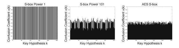
Fig. 4. Confusion coefficients for  $S_1$ ,  $S_{101}$  and  $S_{254}$
