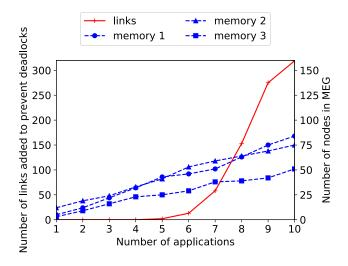
Fig. 5. In red (continuous line), it is shown the number of links that are added to prevent deadlocks as a function of the number of applications (memory size 64 KB per PE). Blue (dashed) curves show the size of MEGs for three memories, as a function of the number of applications.
