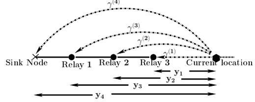
Fig. 5. Measurement-based sequential relay placement. When standing at the “current location,” the deployment operative, having already deployed Relays 1, 2, 3, makes the power measurements  $\gamma^{(k)}$ , and knows the distances  $y_k$ .
