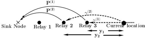
Fig. 6. Sequential deployment with  $n = 2$ . When standing at the “current location,” the deployment operative, having already deployed Relays 1, 2, and 3, measures the powers  $\gamma^{(1)}$ ,  $\gamma^{(2)}$ , and knows the distances  $y_1$ ,  $y_2$  and the lengths  $P^{(1)}$ ,  $P^{(2)}$  of the shortest paths from relay 3 and relay 2 to the sink.
