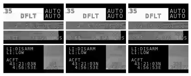
Fig. 9. Reconstruction artifacts for the class-A grayscale-0 decoded video at QP=50. Left: HEVC; Center: SCC; Right: our proposed scheme.
