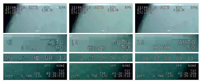
Fig. 8. Reconstruction artifacts for the class-A color decoded video at QP=50. Left: HEVC; Center: SCC; Right: our proposed scheme.
