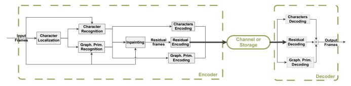
Fig. 2. Architecture of the proposed scheme for encoding airplane cockpit video at low bitrates: the semantics of computer generated graphics (text, lines) are relayed to the decoder separately from the compressed residual video.
