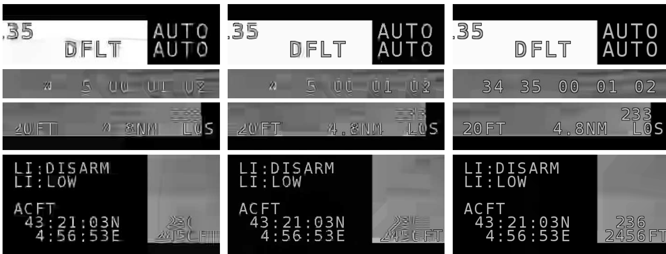
Fig. 9. Reconstruction artifacts for the class-A grayscale-0 decoded video at QP=50. Left: HEVC; Center: SCC; Right: our proposed scheme.
